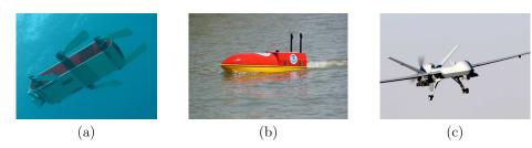
Figure 1.9: (a) The Aqua2 underwater swimming robot from McGill University. (b) A Hydronalix robotic boat. (c) The MQ9 Reaper Unmanned Aerial Vehicle (UAV).
