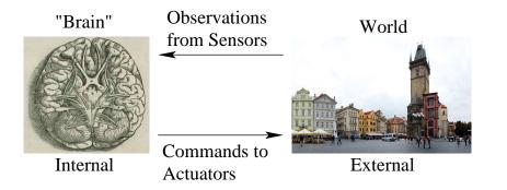
Figure 1.16: In the design of a mobile robot, we erect a boundary between internal and external realms. Information comes from the external, physical world via sensors that produce observations. Commands are transmitted to the external world that cause wheels to roll, legs to walk, and so on. The "brain" holds the information state (I-state), upon which the commands are based.
