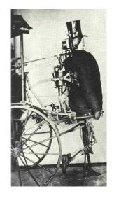
Figure 1.1: In 1868, a "Steam Man" was patented. Its torso was the boiler and its body was mounted upright onto a carriage. Using legs it could walk and steer while pulling a load in the carriage. It is rumored that US President Ulysses Grant once rode in the carriage, called the "Devil's Car".
