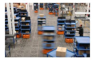
Figure 1.11: An army of Kiva mobile robots moving shelves of boxes in a warehouse.
