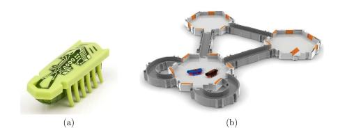
Figure 1.13: (a) A Hexbug Nano. (b) A habitat in which they can navigate along corridors and through rooms. More recent versions include one-way doors and uphill ramps that serve as escalators.
