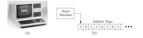
Figure 1.14: Computation models far form mobile robotics: (a) The TRS "Trash" 80, a fine example of classical computing. (b) A Turing machine, which can be imagined as a finite state machine that can read and write bits to an infinitely long tape.
