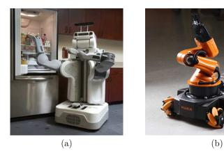
Figure 1.8: Mobile manipulators: (a) The PR2 from Willow Garage. (b) The Kuka Youbot.
