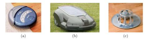
Figure 1.12: (a) A Roomba vacuum cleaner by iRobot. (b) A lawn mowing robot by Husqvarna. (c) The RoboMop floor duster.
