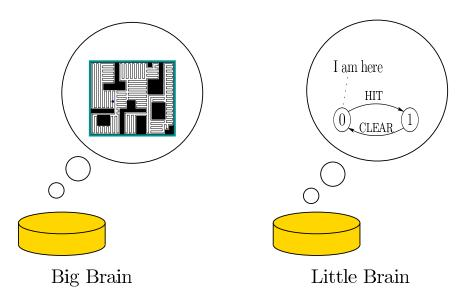
Figure 1.22: What robots are thinking. The big-brain robot maintains a full map of the environment and its own location in the map. The little-brain robot switches between only two I-states.
