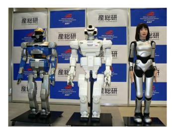
Figure 1.6: The HRP-4 humanoid robots produced in Japan by National Institute of Advanced Industrial Science and Technology (AIST) and Kawada Industries.
