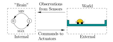
Figure 1.17: Compare to Figure 1.16. The external world is reduced to a robot that rolls along a track, capable of moving only from side to side. On each side is an independent mechanical bumper that senses whether the end of the track as been hit. A "bit brain" that solves the task of patrolling back and forth is merely a two-state machine (also called an automaton).
