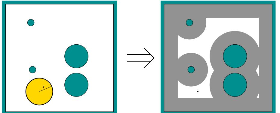
Figure 3.15: If the robot is not a point, then the free space depends in a complicated way on the robot configuration. In the case of a disc-shaped robot of radius  $r$ , it must keep its center at least distance  $r$  from the obstacles.
