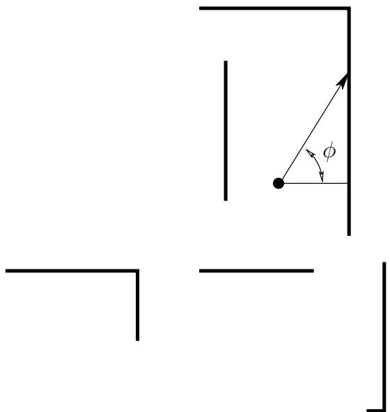
Figure 3.20: For Sensor 8, a function  $y : S^1 \rightarrow [0, \infty)$  is obtained in which each  $y(\phi)$  is the depth in the direction  $\theta + \phi$ . The figure shows how the depth data appears for the environment in Figure 3.19(a) and  $\theta = 0$ .
