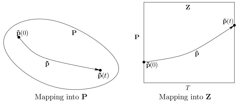
Figure 3.34: A trajectory can be viewed as a time-parametrized path through  $\mathbf{P}$  or a one-dimensional set that traverses  $\mathbf{Z}$  from left to right.
