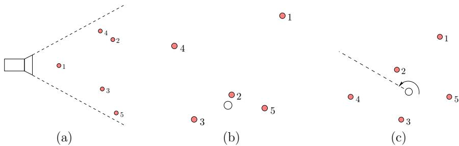
Figure 3.28: Three kinds of compound relational sensors: (a) The linear sensor observes that the landmarks are ordered from left to right as  $(4, 2, 1, 3, 5)$ . (b) This sensor sorts the landmarks closest to farthest, resulting in the observation  $(2, 3, 5, 4, 1)$ . (c) The cyclic sensor sweeps counterclockwise and yields the cyclic ordering  $(1, 2, 4, 3, 5)$
