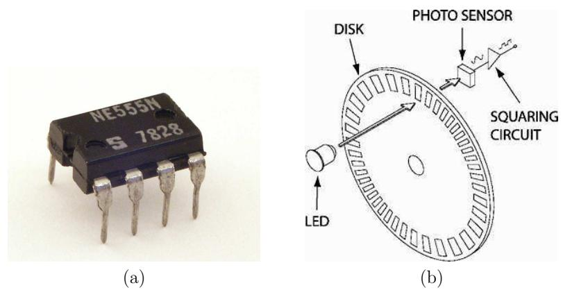
Figure 3.7: (a) The Signetics 555 Timer, one of billions in existence. (b) An optical wheel encoder, to digitally calculate the amount of rotation.
