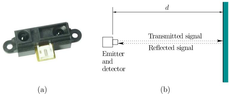
Figure 3.3: (a) The SHARP GP2D120 (around \$12 US), a typical infrared range sensor used on mobile robots. Its published range is between 4cm and 30cm. (b) Most range sensors work by the reflection principle. A signal is transmitted to the obstacle, and the distance is judged based on the reflected signal.
