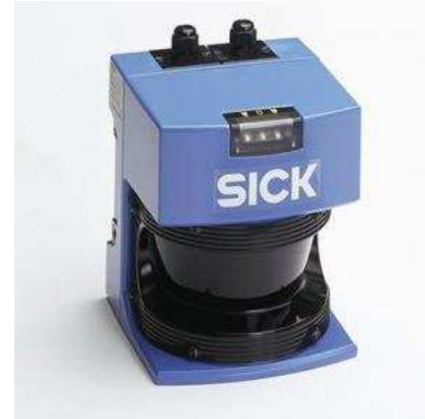
Figure 3.5: The SICK LMS 200 laser scanner, available since the 1990s, provided dense, accurate measurements by beaming the laser into a rapidly rotating mirror.
