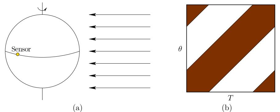
Figure 3.35: (a) Imagine placing a light sensor at an unknown location along the equator of a rotating planet. (b) The sensor preimages partition  $\mathbf{Z}$  into light and dark regions that combine both location and time information.
