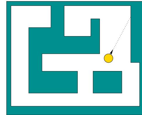
Figure 3.11: A mobile robot is placed in an indoor environment with polygonal walls (more generally called obstacles). It measures the distance to the wall in the direction it is facing.
