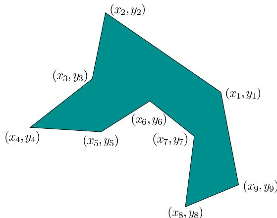
Figure 3.13: A polygonal obstacle is defined by listing its vertices in circular order.
