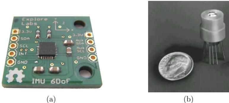
Figure 3.8: (a) Inertial measurement units (IMUs) have been used for decades for tracking aircraft orientation. Nowadays, IMUs are made from microelectromechanical systems (MEMS), resulting in tiny, affordable sensors that are used in smart phones. Pictured is the Explore Labs breakout board for the InvenSense IMU (the black square), which costs around \$50 US. (b) The Dinsmore 1490 compass senses eight quantized directions and costs around \$14 US.
