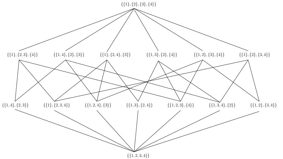
Figure 3.24: The partition lattice for a four-element set. The best and worst sensors are at the top and bottom, respectively.
