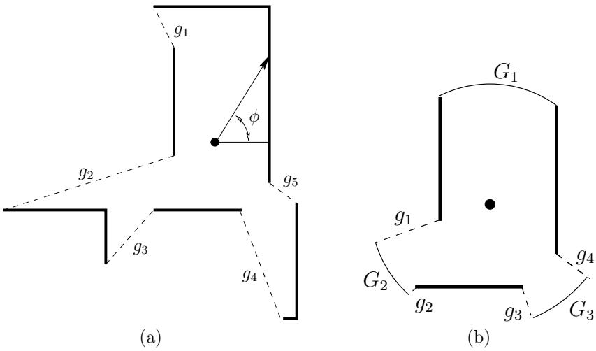
Figure 3.29: Gap sensor models: (a) Five discontinuities in depth are observed. (b) Two kinds of gaps are obtained for a sensor that has limited range.
