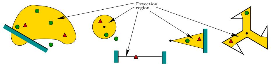
Figure 3.25: A detection region  $V$  is a subset of the free space in which moving bodies (shown as triangles and discs) are detected. Five examples are shown. The detection regions may appear in various shapes and may or may not be attached to a movable body.
