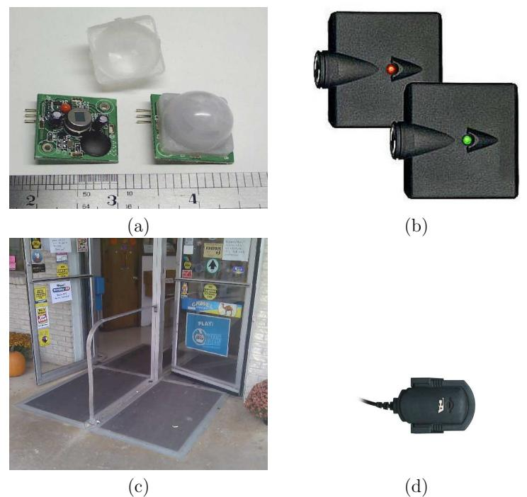
Figure 3.9: Examples of external sensors: (a) A passive IR occupancy detector, often found on ceilings. (b) A Genie garage door detection beam. (c) A supermarket pressure mat, used to determine whether to open the doors. (d) A PC microphone.
