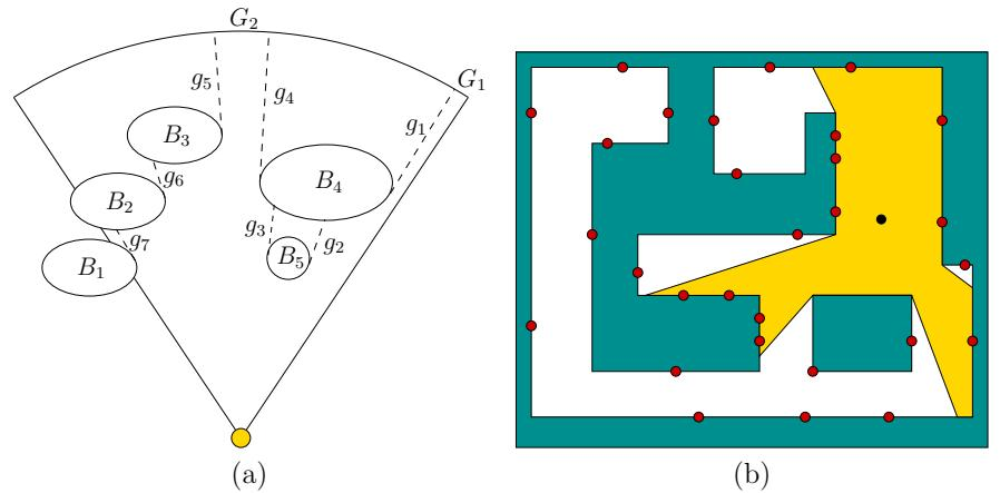
Figure 3.30: (a) A gap sensor among multiple bodies. (b) A sensor that counts landmarks between gaps.
