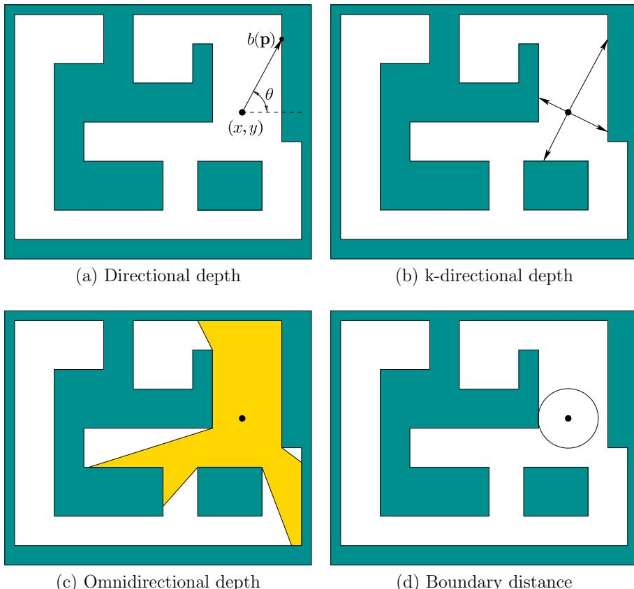
Figure 3.19: Several alternative scenarios for depth sensors.
