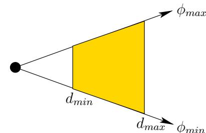
Figure 3.21: A depth sensor that has limited range and angle.
