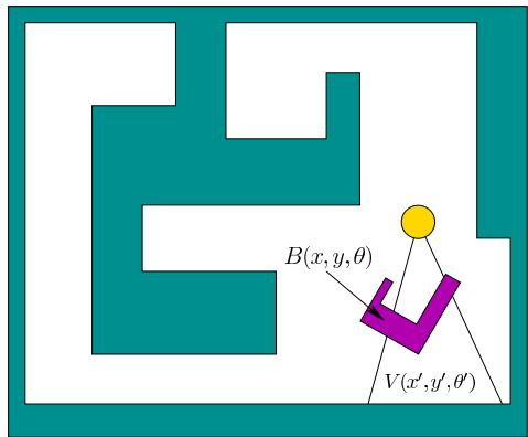
Figure 3.26: For larger bodies, we must declare either *some* or *all* of the body must be in view to be detected.
