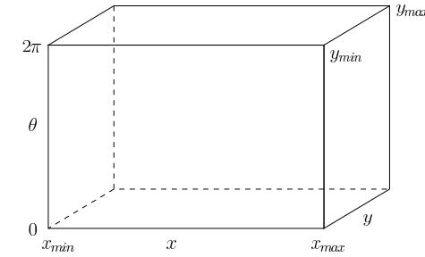
Figure 3.12: With upper and lower limits on  $x$  and  $y$ , The P-space for a planar mobile robot looks like a solid rectangular box. Note that the top and bottom of the box are identical due to the wraparound of  $\theta$  at 0 and  $2\pi$ .
