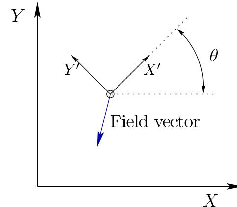
Figure 3.33: If the sensor is rotated by  $\theta$ , then the observed field vector  $f(x, y)$  is rotated by  $-\theta$  with respect to the coordinate system in which the field is defined. To recover the vector in this frame, it must be rotated by  $\theta$ .
