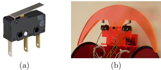
Figure 3.2: Contact sensors: (a) A limit switch closes the electrical circuit when sufficient force is applied to the arm. (b) A bumper attached to the front of a SERB mobile robot built at the University of Illinois. The bumper pivots about a center pin, enabling it to press one of two limit switches, depending on whether the robot hits the obstacle from the left or right corner. (c) The contact sensor from the Lego Mindstorms NXT robotics kit.
