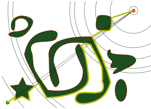
Fig. 1. The robot starts at the lower-left green dot and moves towards the upper-right red dot while traversing various obstacle boundaries. Level sets of equal intensity are represented by the circular arcs.
