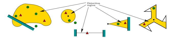
Figure 8: The detection regions may take many different shapes and may or may not be attached to a movable body.
