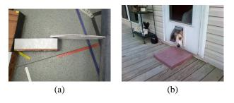
Fig. 7. a) A static, directional gate can be implemented making a flexible "door" from a stack of paper; in this case, the body can transition only from the bottom region to the top; b) this works much like a "doggie door".
