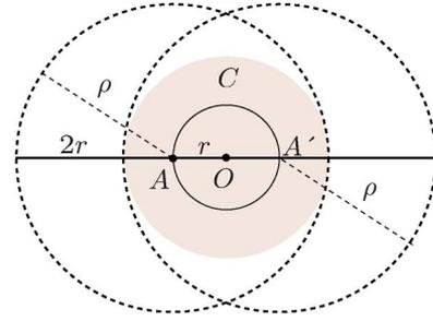
Fig. 12. Agent at  $A$  turns along a circle with center  $O$  of radius  $r$ , leaving the small solid circle as its trace. The two large dotted circles are of distance  $\rho$  to the agent at  $A$  and  $A'$ . The shaded disc denotes the intersection of all discs with radius  $\rho$  from the agent as it turns a full cycle.
